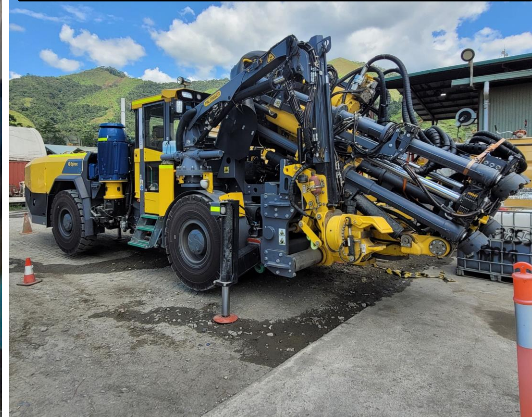
Epiroc Easer L Raise Bore – Arrived on Site Late-July
